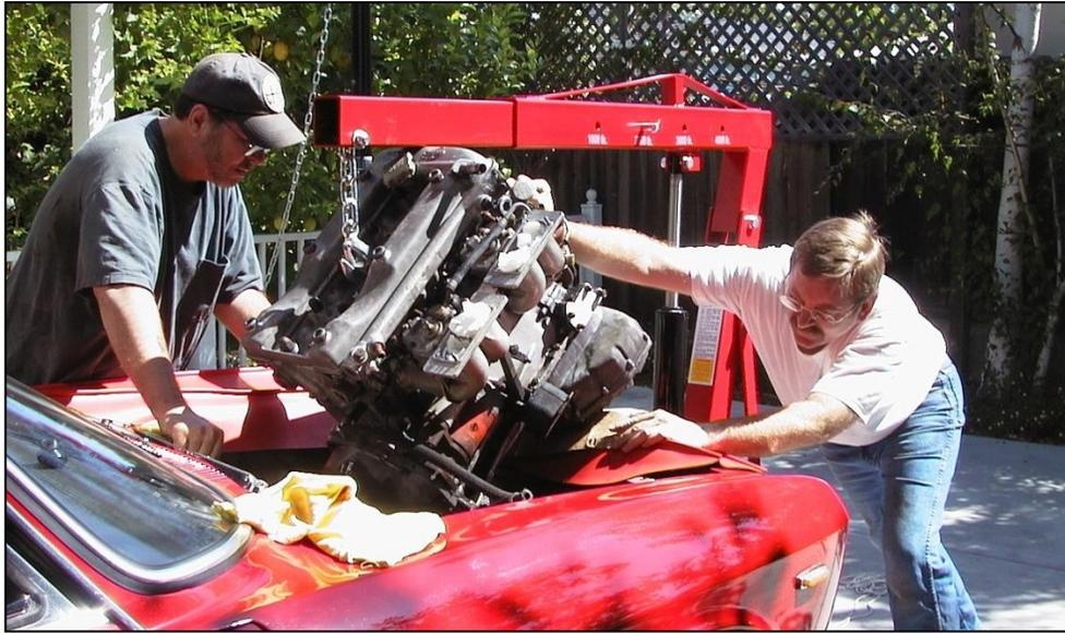
Gary, left, and friend Steve Smith pull a 1750 engine prior to replacing it with pumped 2L, circa 2005.
