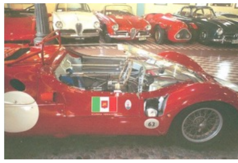
1960 Maserati Tipo 63 "Birdcage" with mid-engine V12. Chassis composed of over 200 pieces of welded steel tubing, creating a space-frame weighting only 36 kg (80 lbs).
