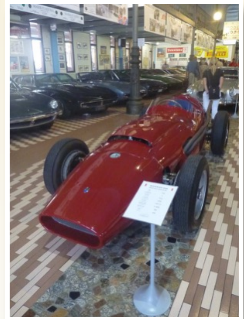
1957 Maserati 250F Prototype, driven by Fangio, did not qualify at Monaco GP due to engine failure; dual overhead cam in-line six, 2.5 liter, 240 hp.
