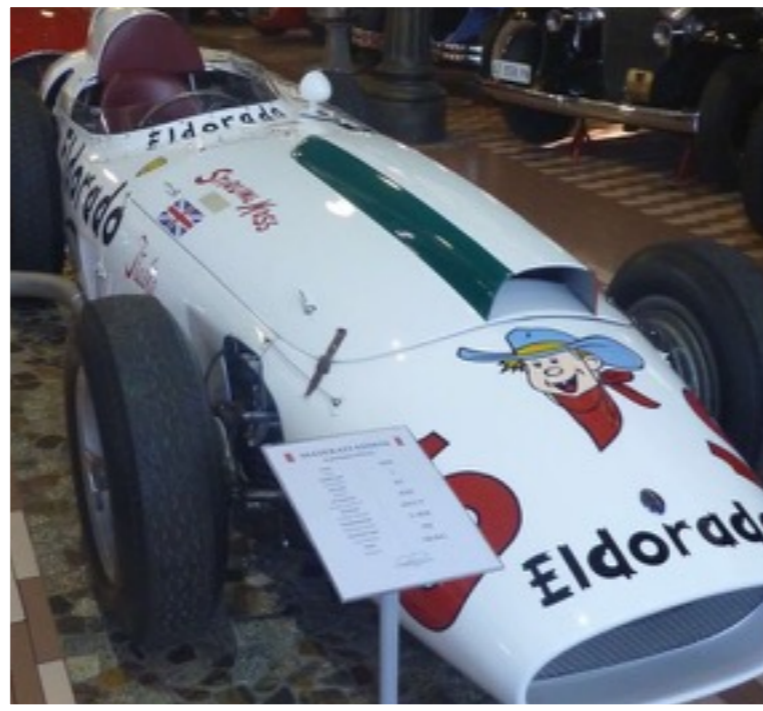
1958 Maserati 420M, specifically built for 500 miles of Monza (Monzanapolis), driven by Sterling Moss; dual overhead cam in-line six, 4.2 liter, mix of 250F and 450S components. First European race car to be sponsored by non-automotive sponsor.
