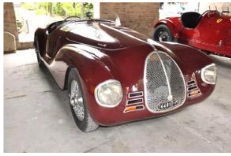
Righini AAC815 AscariMM: 1939 Auto Avio Costruzioni Tipo 815 Spider, 1.5 liter straight eight, body by Touring. This was one of two of Enzo Ferrari's first constructed cars.
