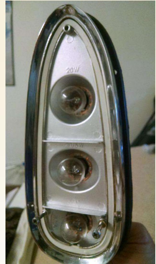
OEM 9" 101 series tail light assembly restored. New tail light to body mounting gasket, a new lens gasket, all new SS hardware, and all new light bulbs. The lens is useable, though not pristine. One may notice that the signal portion of the lens isn't amber, it's red. It's the original stock lens.
